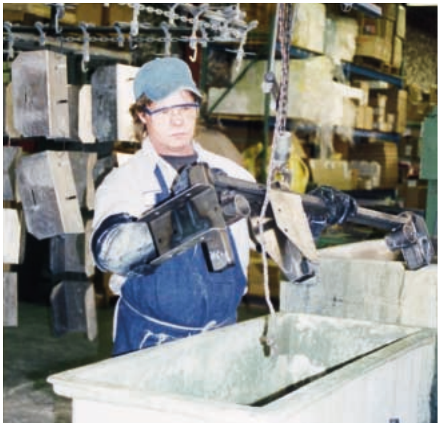
Rand-Scot associate Jim Murphy loads an EasyPivot frame into the metal treatment product's tank for pretreatment.
