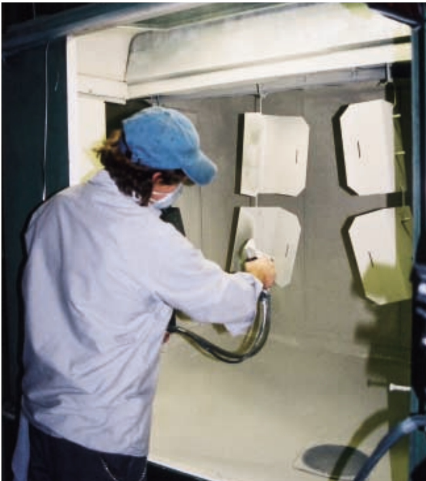
An operator applies a triglycidyl isocyanurate-based polyester powder coating to brackets for the EasyPivot lift.
